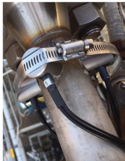
XD-301 attached with hose clamp
