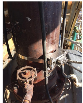
XD-201 probes attached with clamp
