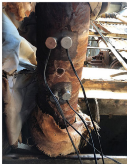
XD-301 attached with magnets
