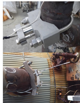
XD-201 attached with U-bolt
