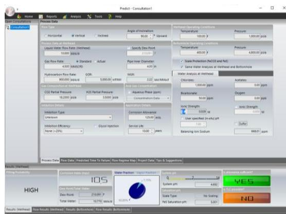
Predict main program interface, showing predicted carbon steel corrosion rate, pitting corrosion likelihood and other relevant results
