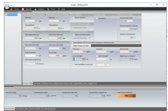
Top of the Line Corrosion – evaluate TLC corrosion rate, condensation rate and condensed water pH as a function of operating conditions.
