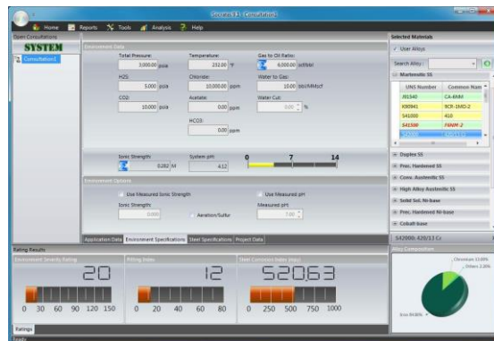
Socrates' program interface shows a list of acceptable materials based on specified environmental conditions and application requirements
