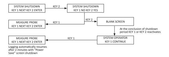
To activate the system shutdown function, the user should scroll through the main function screens using KEY 1 until the "SYSTEM SHUTDOWN" function screen is reached. The user can now use KEY 2 to access the submenu. The screen will now ask for confirmation. KEY 2 will activate system shutdown; KEY 1 will return the user to the main function screens. If KEY 2 is used to activate "SYSTEM SHUTDOWN", data logging will cease but all existing data will be retained in memory.
