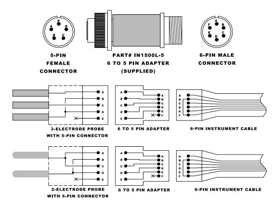
In some cases the user may encounter probes with non-standard wiring. In this case a custom adapter may be required. Alternately the IN1500L-4 flying lead adapter (sold separately) may be used. The IN1500L-4 consists of a standard instrument-end connector, while the probe-end terminates in flying leads with alligator clips. This allows the user to make connections as required for non-standard probes.
