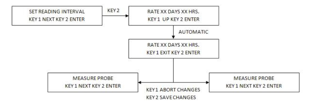
After any key is used to activate the screen, KEY 1 is used to scroll to the "SET READING INTERVAL" main function screen. KEY 2 then allows entry into the submenu.
