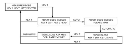
The first screen of the "MEASURE PROBE" submenu displays the probe I.D. number and measurement type. KEY 1 exits to the main menu "MEASURE PROBE" function screen and KEY 2 will activate a measurement.
