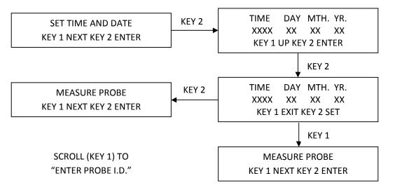
The screen of the instrument is initially activated by pressing either key. The "SET TIME & DATE" function screen is then accessed by scrolling through the main menu using KEY 1. KEY 2 allows entry into the submenu, and the time and date setup screen will be shown. Each digit of the time, day, month, and year is sequentially set using KEY 1 to select the appropriate digit, and KEY 2 to enter the digit and move the next digit of the time and date sequence.
