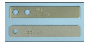
**Scale coupons** (or deposition coupons) provide a qualitative measure of relative deposition rates in industrial water and manufacturing process systems.
