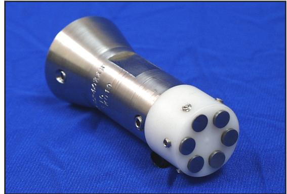
The main problem with this approach is that most of the harmful species of bacteria (sulfate reducers) are sessile and grow as colonies on the internal surfaces of the pipeline or vessel. Bulk fluid samples only provide information on those bacteria which are “in the flow” and not apt to cause damage. Therefore to help prevent significant damage before it can occur, pipe wall monitoring is needed which can show signs of biological activity when the colonies are established.
