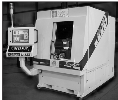
Photo 1 – Example of a laser metal deposition system.
