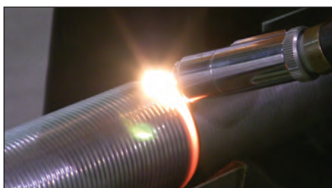
Boiler tubes (alloy steel) clad with Alloy 622
