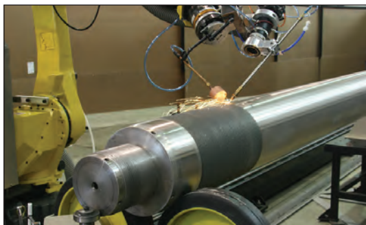
Hydraulic shaft clad for corrosion resistance
