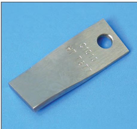
P/N CO303 Twist Specimen
