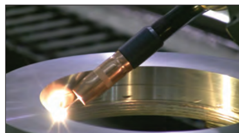
Repairing damaged areas to oil & gas seat
