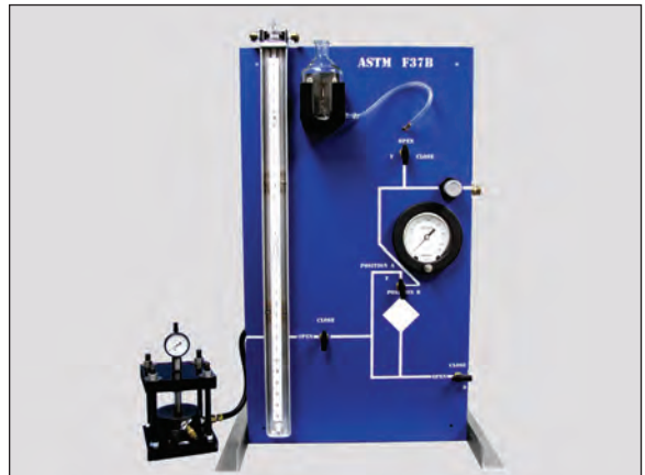
ASTM F37 (Method B) Test Cell with Test Panel. This is the complete assembly for the ASTM F37 (B) test method. Assembly is ready for attachment to pressure supply.
