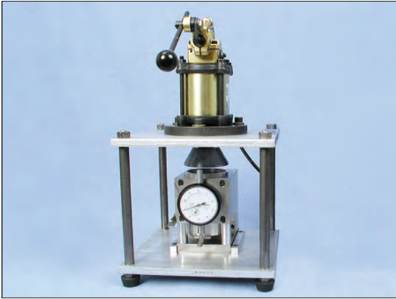
ASTM F36 Test Cell for compressibility and recovery of gasket materials. Fixture shipped partially assembled.
