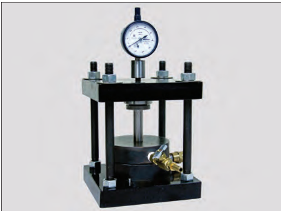
ASTM F37 (Method B) Test Cell is used to evaluate the gas sealability of gasket materials. This test cell can also be used for evaluating liquid sealability.
