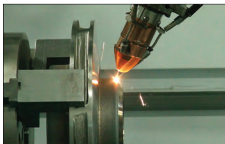
Flanges (stainless steel) clad with Alloy 625 to enhance erosion / corrosion resistance (Left: before machining, Right: after machining)
