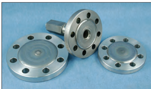
Flanges (stainless steel) clad with Alloy 625 to enhance erosion / corrosion resistance (Left: before machining, Right: after machining)
