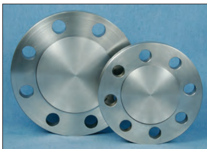
Flanges (stainless steel) clad with Alloy 625 to enhance erosion / corrosion resistance (Left: before machining, Right: after machining)
