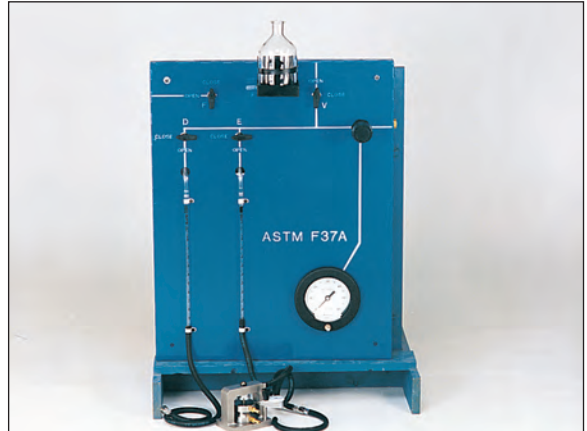
ASTM F37 (Method A) Test Cell with Test Panel. This is the complete assembly for the ASTM F37 (A) test method. Assembly is ready for attachment to pressure supply.
