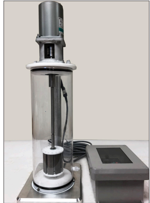
Atmospheric Pressure Rotating Cage to Evaluate Corrosion Inhibitors in the Oil and Gas Industry
