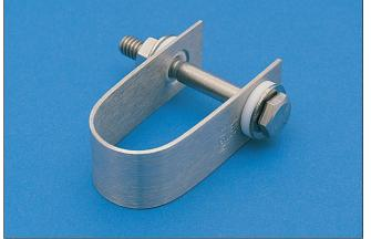
P/N TF2404 Stressing Frame with P/N TF2447 4-Point Bent Beam Assembly - ASTM G39
