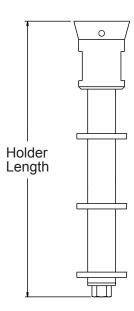
Figure 6. Multiple Disc Coupon Holder
