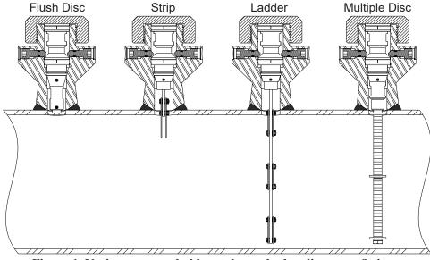
Figure 1. Various coupon holder styles on hydraulic access fittings.
