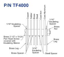
**ASTM D1384** corrosion test bundle for testing engine coolants in glassware.
