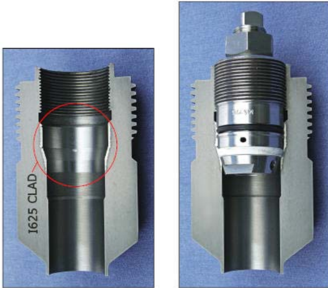
Figure 2: Cladding of I625 alloy only for the seal seat
